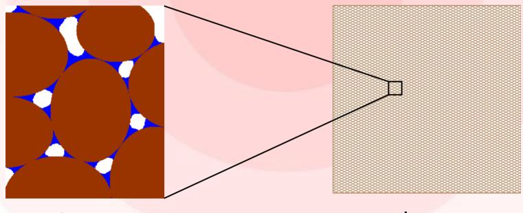
micro-scale: non-homogeneous  $\lambda(x)$  macro-scale: homogeneous  $\lambda_e$
